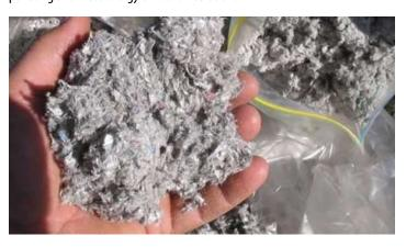
Cellulose has the highest post-consumer recycled content. The fiberglass industry averages 35% recycled glass, while the cellulose industry averages a minimum of 75% recycled content. It takes more than 10 times as much energy to produce fiberglass insulation as cellulose insulation.
